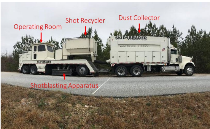
(a) Shotblasting System
