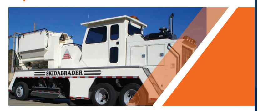
SKIDABRADERS patented high velocity, bi-directional impact method uses multiple blast wheels propelling steel abrasive at the surface in a proprietary head design. These 1000 horsepower units can texture 360 degrees around the aggregate to provide improved micro and macro texture. Skidabrading is the fastest and most economical method to address friction requirements and re-texturing on roads and runways with infinite variables to achieve any specification results needed.
