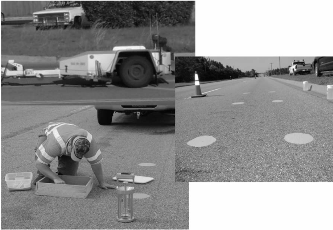
Figure 2. ODOT Skid Trailer, Outflow meter ASTM STP 583 and the Transit New Zealand TNZ T/3 Sand Circle Testing
