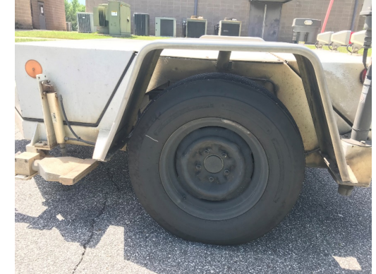
Locked-wheel skid trailer (LWST)
