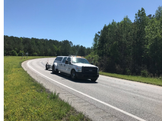
Locked-wheel skid trailer (LWST)
