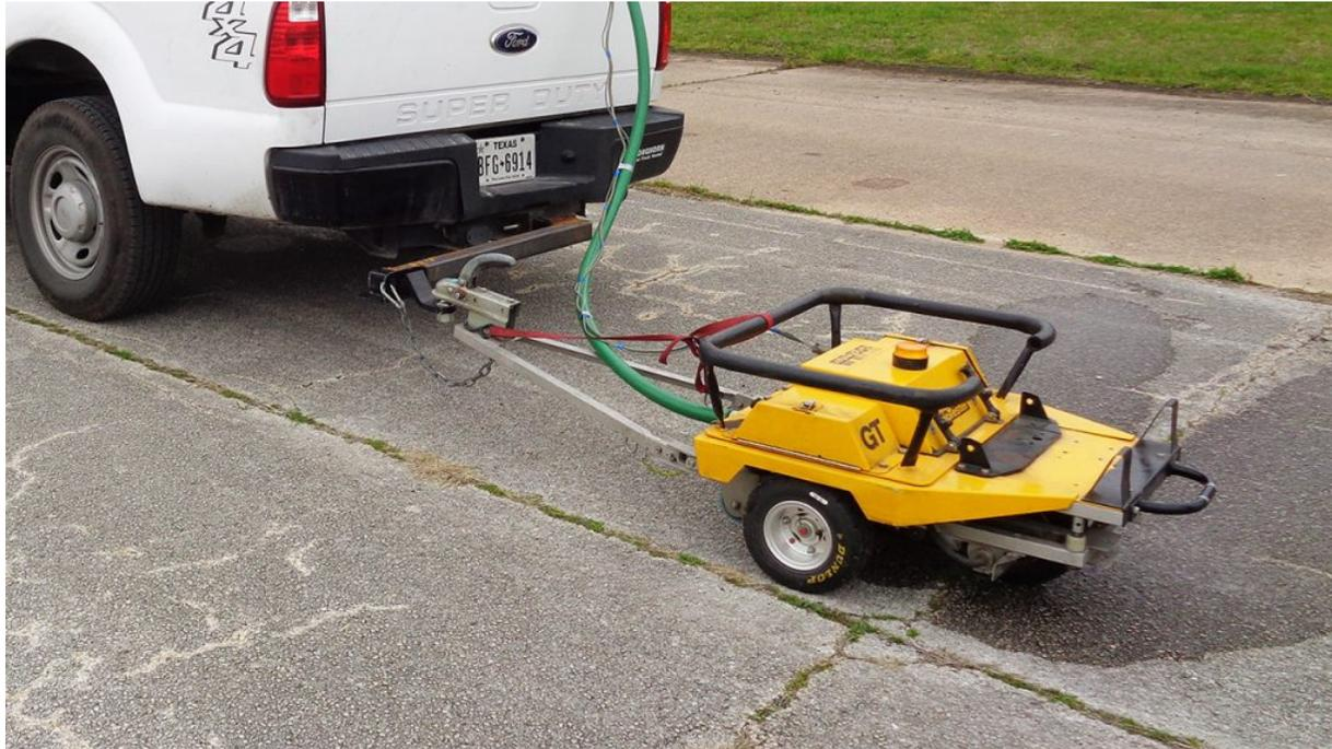
Because wet pavement has lower friction than dry pavement and is considered a worst case, the GripTester contains a self-wetting system which applies a 1 mm (0.04 inch) depth water film just in front of the test tire. For runways, the typical test procedure is to measure friction at speeds of 40 and 60 mph and at 10 and 20 feet on each side of the runway centerline. Results are reported in 500-foot intervals.
