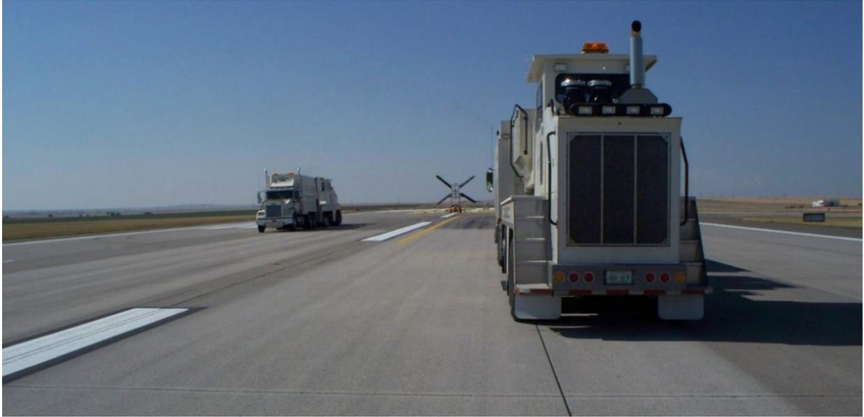
Waterblasting works similar to shotblasting but uses high pressure water instead of steel media. It is generally not as aggressive to the pavement surface as the mechanical texturing process and mainly removes rubber with little additional improvement of macrotexture. With the chemical cleaning method, chemicals are applied to the pavement and then washed off with lower pressure water. The chemicals breakdown the rubber without changing the pavement surface.
