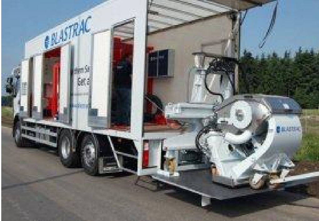
Photo 2 Blasting unit in rear of lorry
