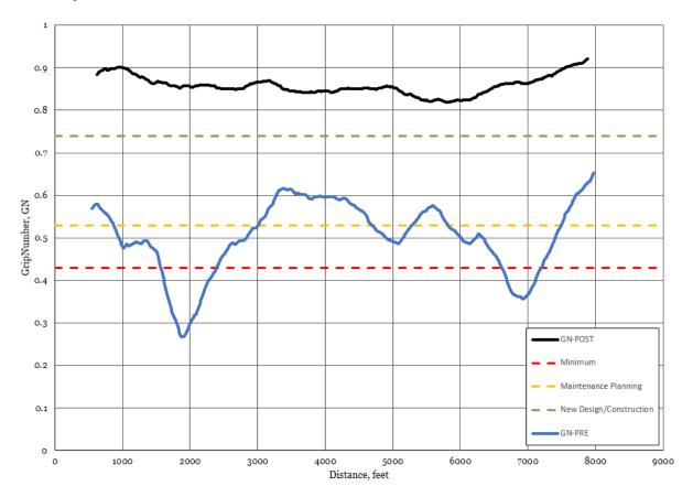
The graph illustrates pre- and post-shotblast friction results on Runway 13R. Post-shotblast friction levels (represented by the solid black line) exceed FAA required minimum levels for new design/construction (represented by the dashed green line).
