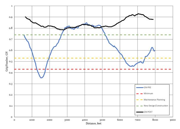
The graph illustrates pre- and post-shotblast friction results on Runway 31L. Post-shotblast friction levels (represented by the solid black line) exceed FAA required minimum levels for new design/construction (represented by the dashed green line).
