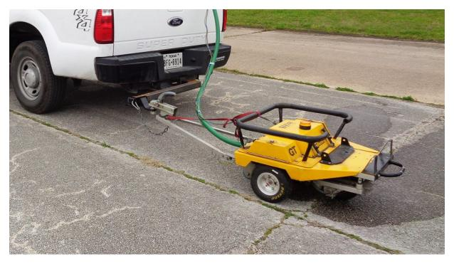
Because wet pavement has lower friction than dry pavement and is considered a worst case, the GripTester contains a self-wetting system which applies a 1 mm (0.04 inch) depth water film just in front of the test tire. For runways, the typical test procedure is to measure friction at speeds of 40 and 60 mph and at 10 and 20 feet on each side of the runway centerline. Results are reported in 500-foot intervals.
